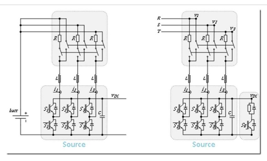
Battery can be connected to same circuit as 3ph PFC!
